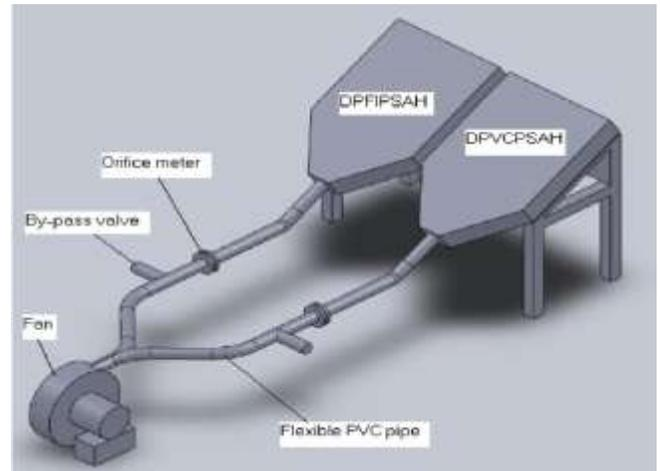
Fig 6: The schematic diagram of the experimental setup is shown above [8]
