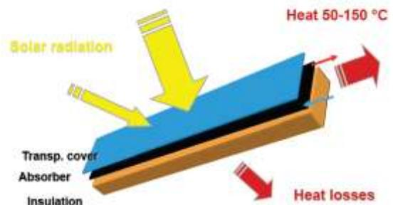
Fig 1: Flat Plate Collector
