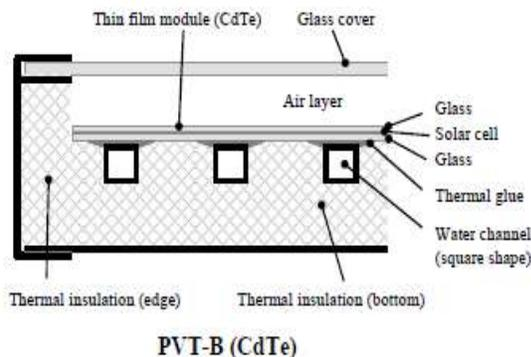
Fig 3: (PVT-B) with CdTe thin film solar cells [1]
