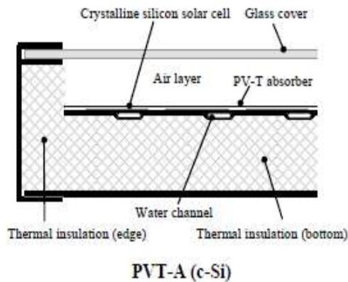
Fig 2: Cross sections of two covered flat-plate PVT water collectors.(PVT-A) with laminated c-Si solar cells [1]
