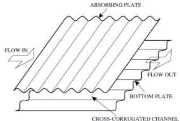
Fig 4: schematic description of corrugated plates of type 1 [2]
