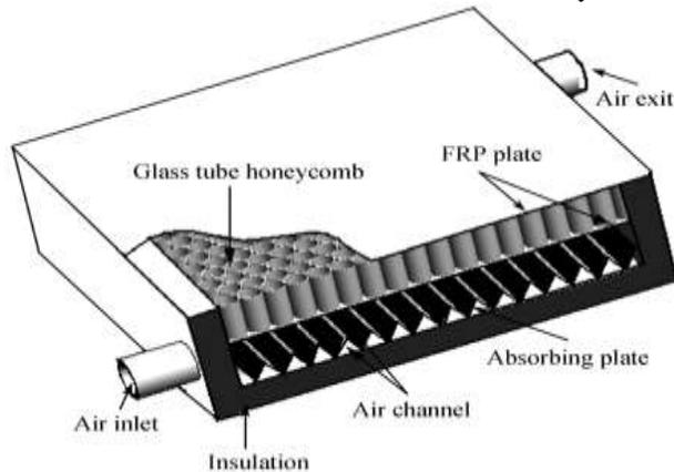
Fig. 5: Honeycomb Structure
